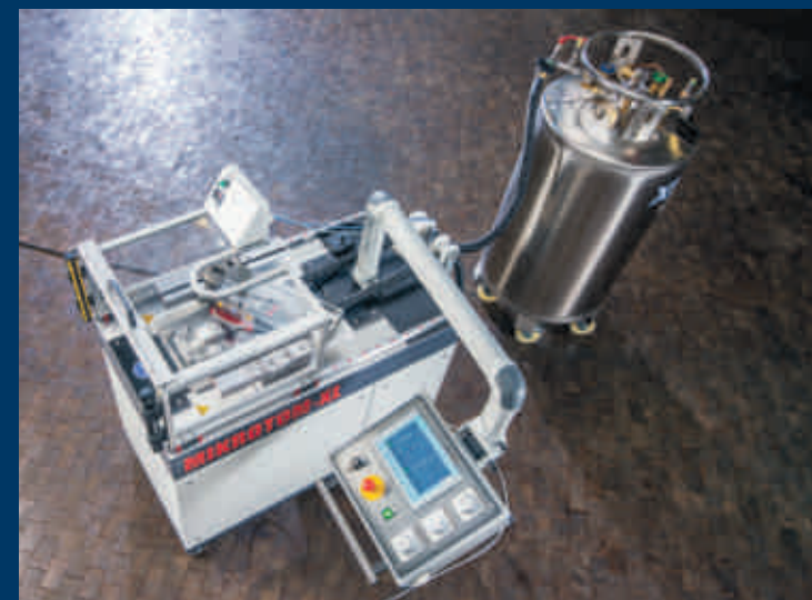
Mikrotom-XL with liquid nitrogen cooling unit and safety housing when in continuous stroke mode
